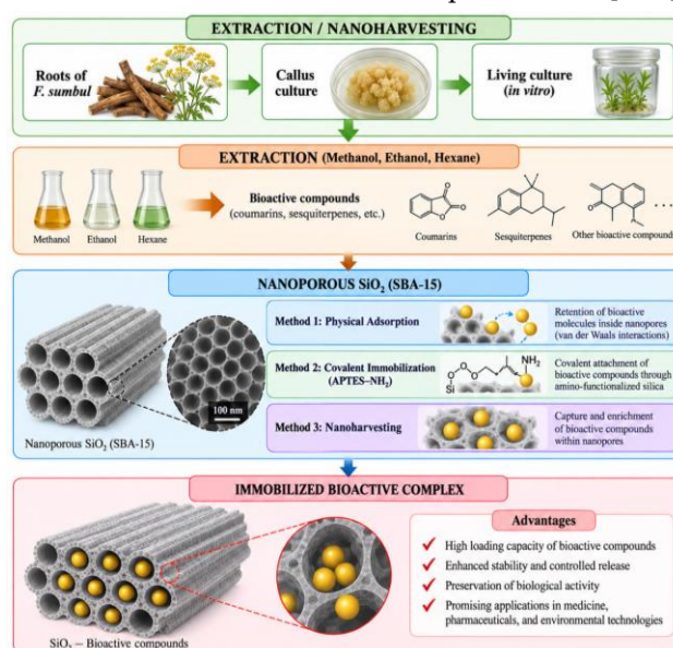
Figure 1. Schematic of the immobilization of Ferula sumbul bioactive substances on nanoporous SiO 2 [7, 16].
