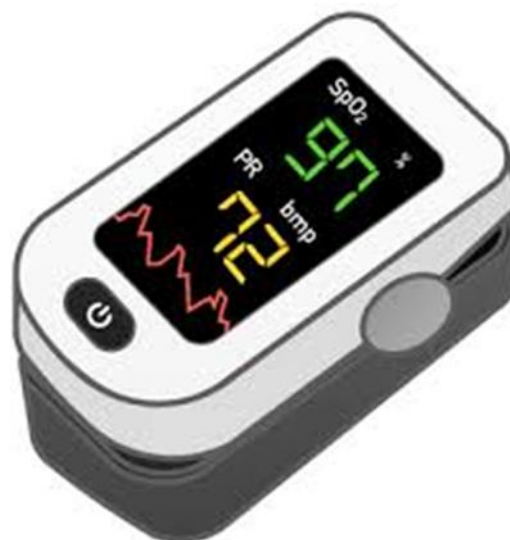
Figure 1. Finger clip pulse oximeter, health monitoring Small package and high functionally integrated MCUIntegrates a sink current generator, a pulse oximeter AFE and an LCD driver. Convenient development Provides program libraries to calculate the blood oxygen saturation level, pulse rate and perfusion index.
