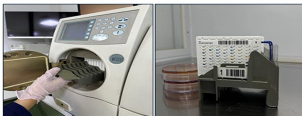
Figure 1. VITEK 2 Compact System and Preparation of Reagent Cards for Antimicrobial Susceptibility Testing.
