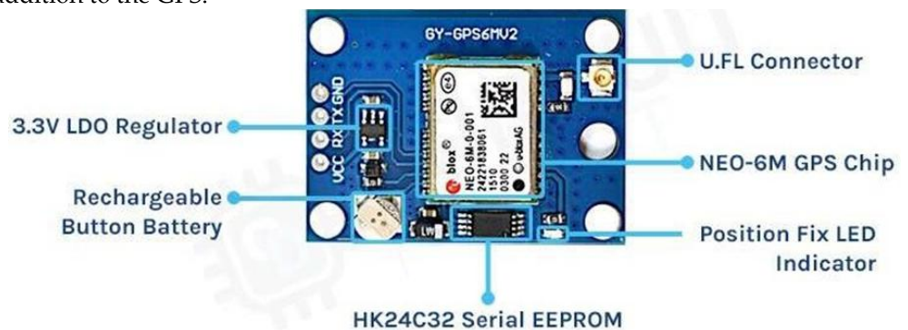
Figure 5. Structure of GPS NEO 6M
