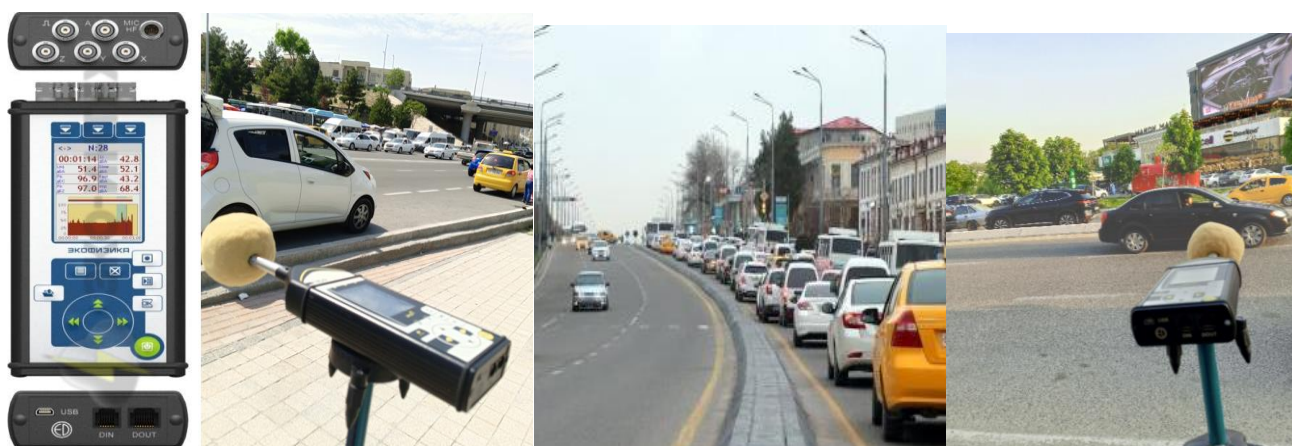
Figure 2. The territory was surveyed using the Ecophysics 110 A device (noise meter)
